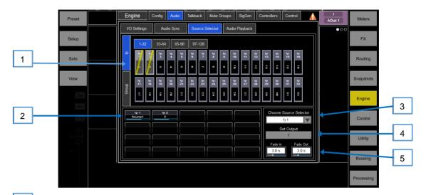
Sources: Inputs / Groups – Use the vertical tabs to switch between inputs and groups. Drag and drop inputs and/or groups into the lower pane to add them to a Source Select group.
