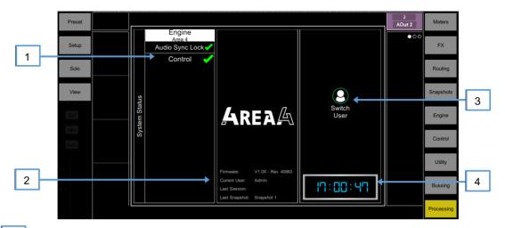
System Status – Displays a list of system components. A green tick indicates the component is running correctly. A red cross indicates that an error is detected. A blue icon appears when a non-critical event is logged. Click the component to display further information.
