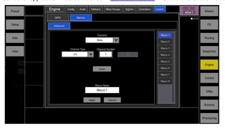
The onboard Engine GPIO ports are configured in Engine/Control/GPIO/Advanced.
