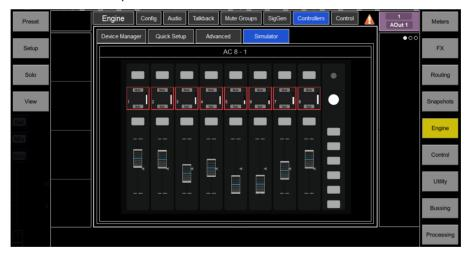
Click a button on the screen to control the assigned function. Click and drag a fader / rotary control to control the assigned parameter.
