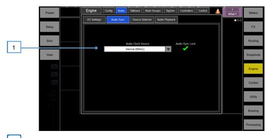
Audio Clock Source – Select the device which should provide audio sync – internal, word clock input or relevant DMI cards.
