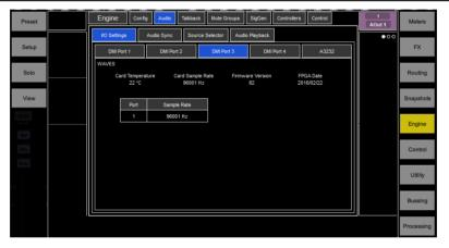
DMI Waves Card will need Soundgrid Network configuration in addition to its **Sync Source** settings. This is done using either Waves MultiRack or SoundGrid Studio, both of which are available from: <a href="http://www.waves.com/downloads">http://www.waves.com/downloads</a>
