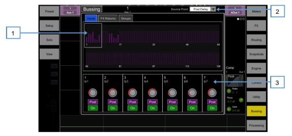
**Aux and FX sends** – Displays routing and assignments of Input channels, FX Returns and Groups to the selected Mix.
