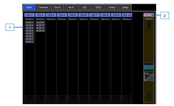
**CGs** – Displays name, members (assigned channels) and whether the 'Fader to Zero dB' option is enabled. Use the **Bussing** screen to assign channels.
