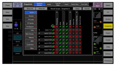
Use the tabs on the left to view the different parameter groups. scroll to zoom in and out of the matrix view. Drag up/down or left/right to navigate through the matrix. Click an item to toggle. Allowed items will be recalled, Blocked items will not.
