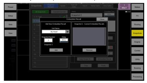
Set the **Snapshot Number** to select the Snapshot you wish to recall. Its name is displayed below the box. Set the **Delay** time for the snapshot recall. This is the time the system waits before recalling the Snapshot after you have recalled the host Snapshot. Time can be set from 0 sec (instant) to 4 minutes. Click **Add** to add the Snapshot to the list on the right.
