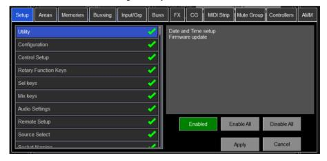
**User permissions** – Each User can have their own set of Permissions applied. Use the tabs across the top of the window to view and set different groups of permissions. Select an item in the list and toggle the **Enabled/Disabled** button as required. The window on the right provides a description of the functions included in the currently selected item. Use the **Enable All / Disable All** buttons to quickly toggle all items in the currently open tab. Click **Apply** to accept the changes.
