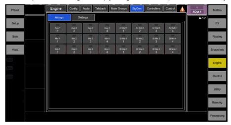
**Assign** – Click a Mix button to assign the SigGen. The signal routes through the Mix processing, therefore will be affected by the Mix EQ and compressor.
