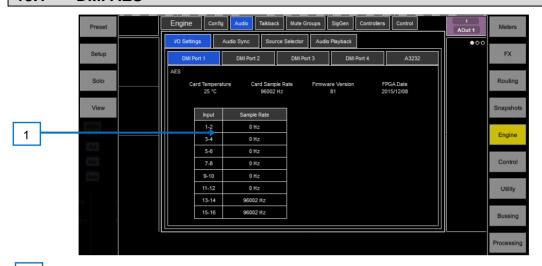
Input SRC Display – Enable the SRC Bypass option in Routing view by clicking on the relevant socket to disable input sample rate conversion on a socket pair basis.
