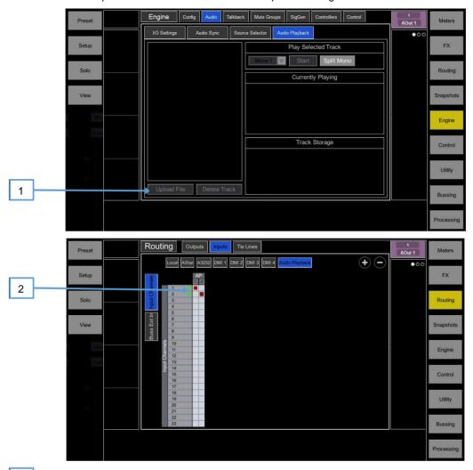
With the Controller computer connected to the 4REA4, click on **Upload File** and select the required audio file from the Controller computer's drive – then follow the on-screen instructions to upload the file.
